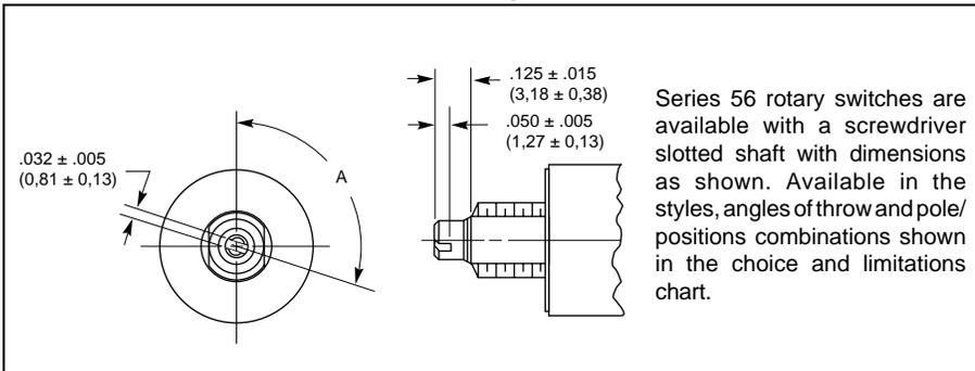
Series 56 rotary switches are available with a screwdriver slotted shaft with dimensions as shown. Available in the styles, angles of throw and pole/positions combinations shown in the choice and limitations chart.
