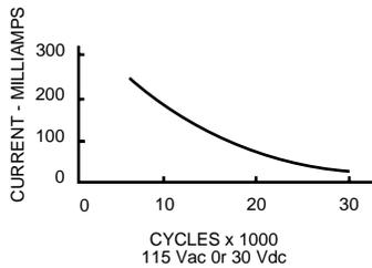
One cycle is 360° rotation clockwise and 360° return. The data for the curve was measured at sea level, 25°C and 68% relative humidity with the life limiting criteria which follows.
