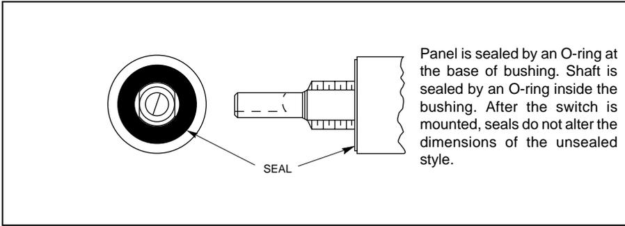
Panel is sealed by an O-ring at the base of bushing. Shaft is sealed by an O-ring inside the bushing. After the switch is mounted, seals do not alter the dimensions of the unsealed style.
