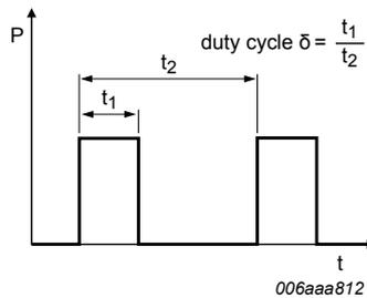
Fig. 18. Duty cycle definition
