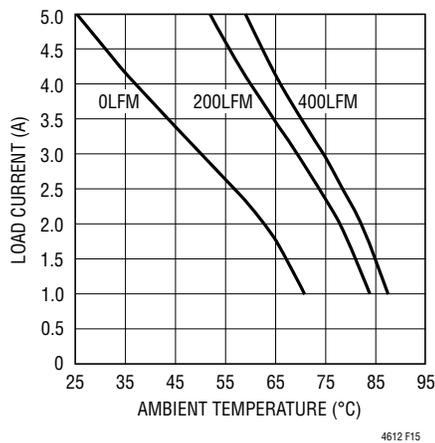
**Figure 15. No Heat Sink with 36V<sub>IN</sub> to 15V<sub>OUT</sub>**
