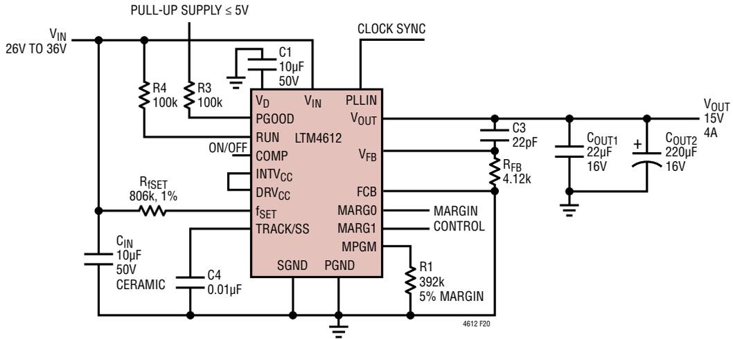
Figure 20. 26V to 36V<sub>IN</sub>, 15V at 4A Design with Reduced Frequency
