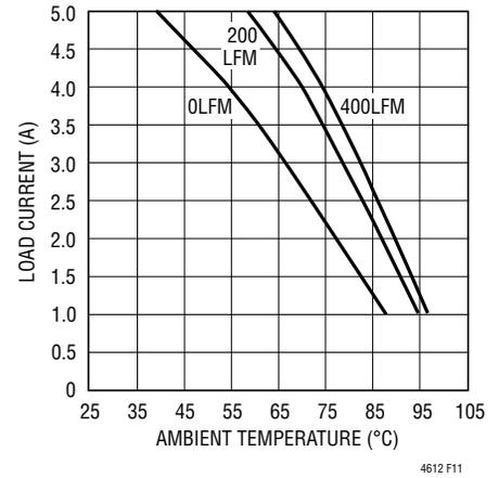
**Figure 11. No Heat Sink with 36V<sub>IN</sub> to 5V<sub>OUT</sub>**
