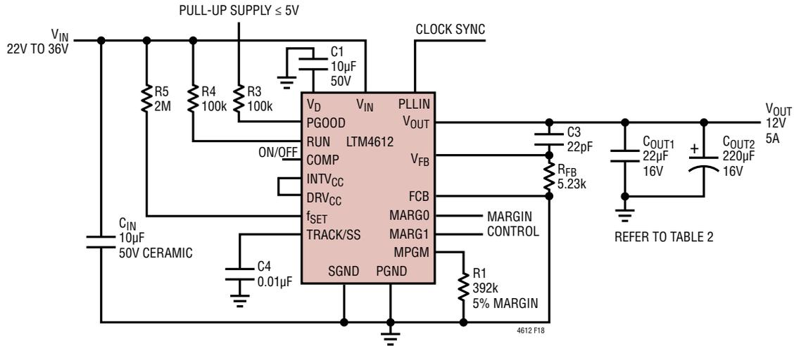
Figure 18. Typical 22V to 36V<sub>IN</sub>, 12V at 5A Design
