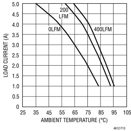
**Figure 13. No Heat Sink with 24V<sub>IN</sub> to 12V<sub>OUT</sub>**
