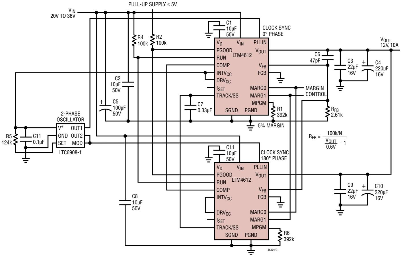
Figure 21. 2-Phase, Parallel 12V at 10A Design
