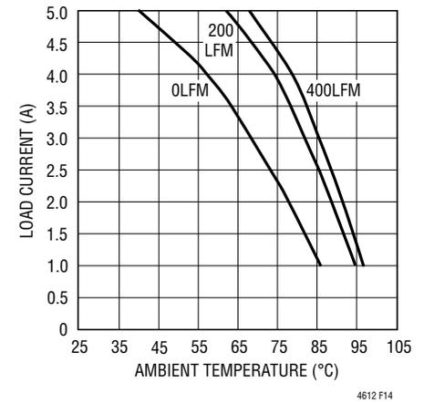
**Figure 14. BGA Heat Sink with 24V<sub>IN</sub> to 12V<sub>OUT</sub>**
