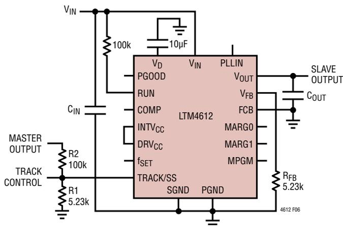
Figure 6. Coincident Tracking
