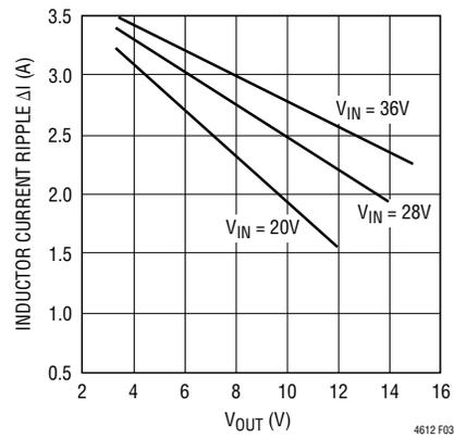
Figure 3. Inductor Current Ripple vs Output Voltage
