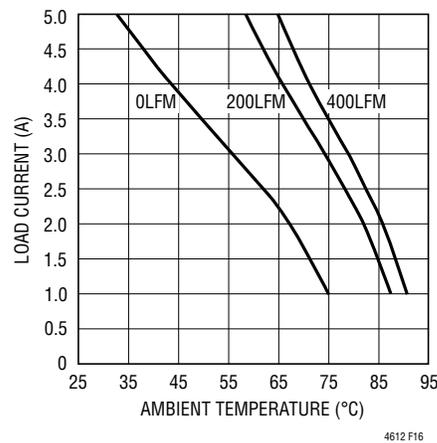
**Figure 16. BGA Heat Sink with 36V<sub>IN</sub> to 15V<sub>OUT</sub>**
