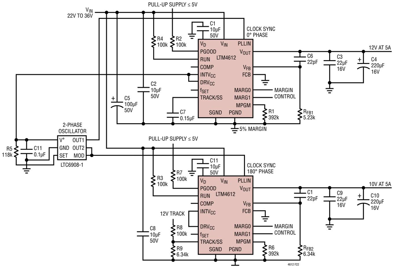
Figure 22. 2-Phase, 12V and 10V at 5A Design
