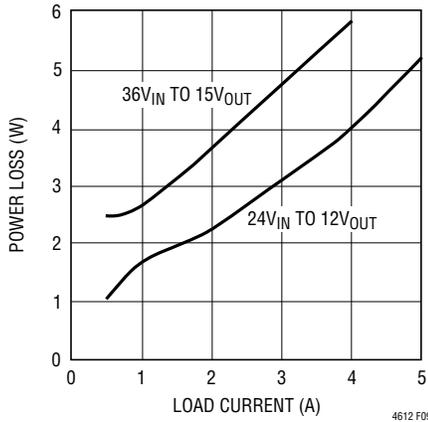
**Figure 9. Power Loss at 12V<sub>OUT</sub> and 15V<sub>OUT</sub>**
