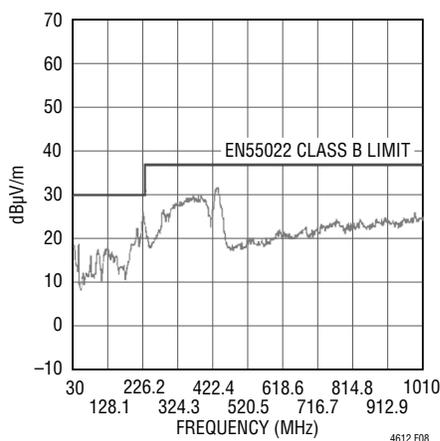
**Figure 8. Radiated Emission Scan with 24V<sub>IN</sub> to 5V<sub>OUT</sub> at 5A Measured in 10 Meter Chamber**
