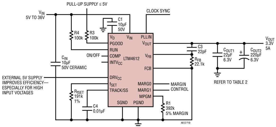
Figure 19. Typical 5V to 36V<sub>IN</sub>, 3.3V at 5A Design with 400kHz Frequency
