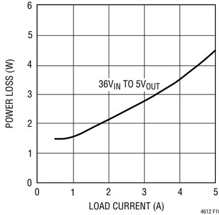
**Figure 10. Power Loss at 5V<sub>OUT</sub>**
