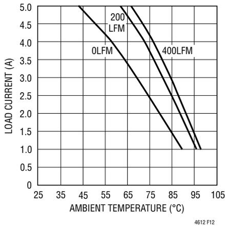
**Figure 12. BGA Heat Sink with 36V<sub>IN</sub> to 5V<sub>OUT</sub>**
