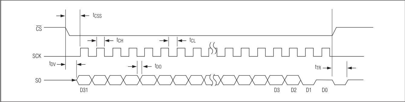
Figure 2. Serial-Interface Timing
