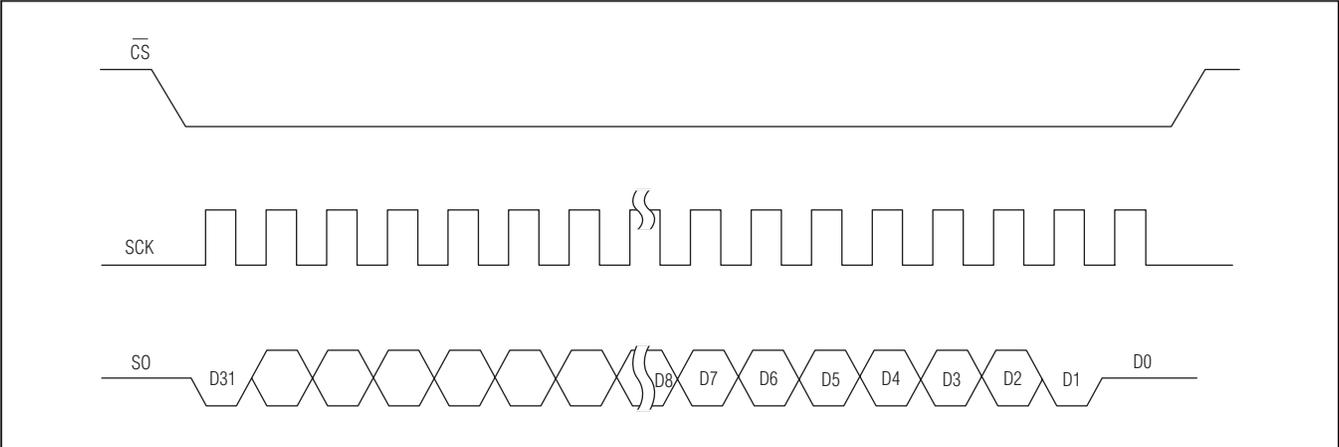
Figure 1. Serial-Interface Protocol
