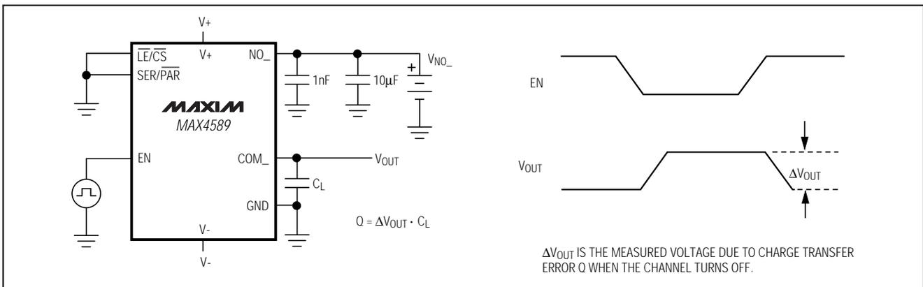
Figure 3. Charge Injection
