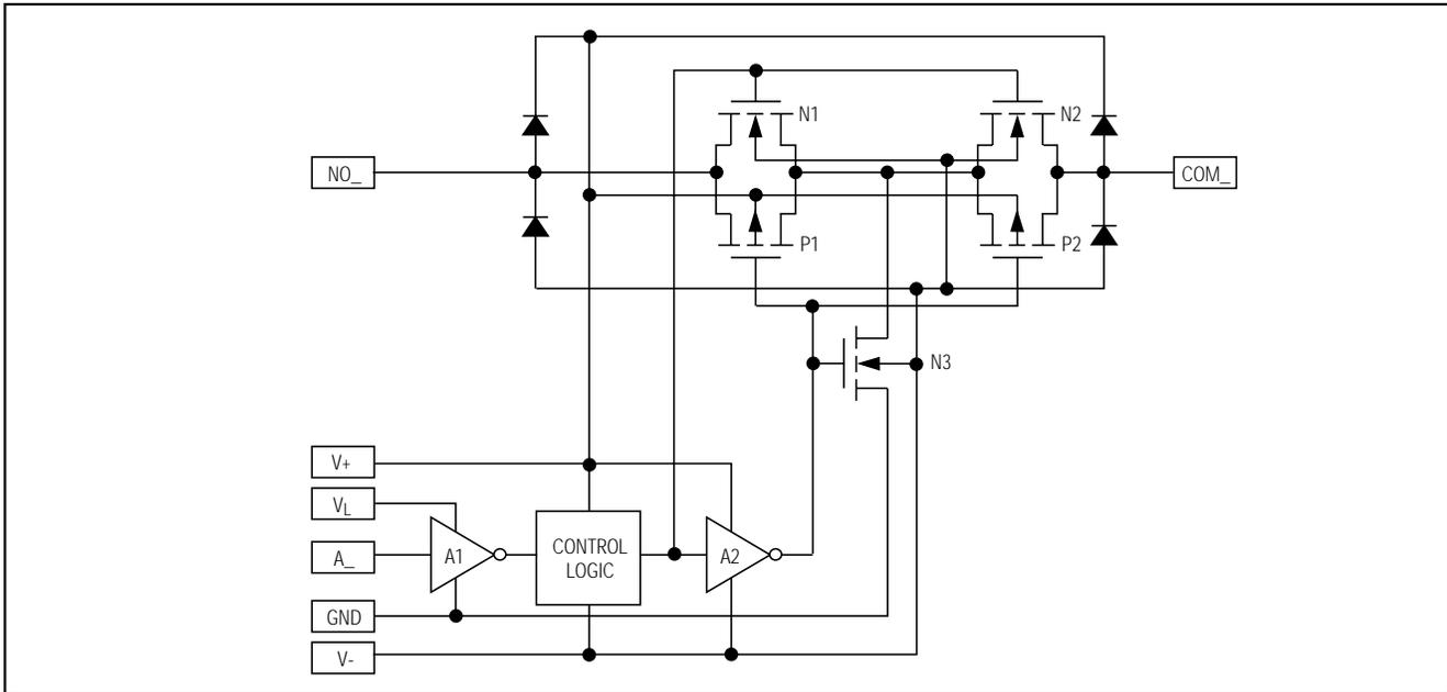
Figure 8. T-Switch Construction
