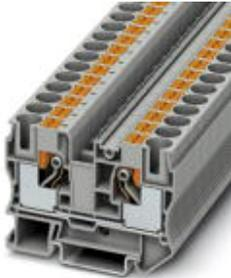
Feed-through terminal block, Connection method: Push-in connection, Cross section: 0.5 mm<sup>2</sup> - 16 mm<sup>2</sup>, AWG: 20 - 6, Width: 10.2 mm, Height: 49.5 mm, Color: orange, Mounting type: NS 35/7,5, NS 35/15
