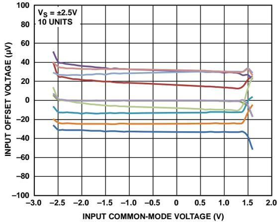
Figure 24. Input Offset Voltage vs. Input Common-Mode Voltage
