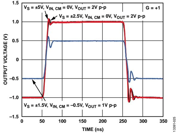
Figure 32. Large Signal Transient Response for Various Supplies
