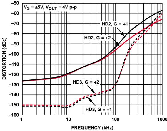
Figure 12. Distortion vs. Frequency for Various Gains
