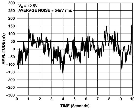
Figure 18. 0.1 Hz to 10 Hz Voltage Noise
