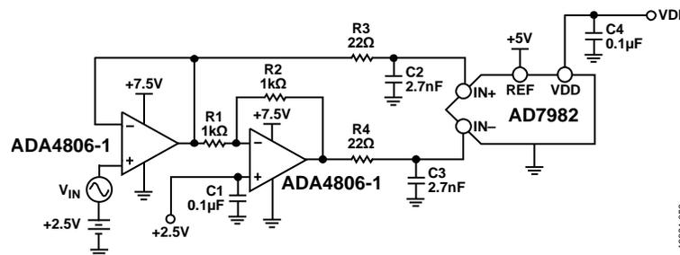
Figure 65. Driving the AD7982 with the ADA4806-1
