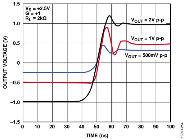
Figure 57. Step Response with Selected Output Steps
