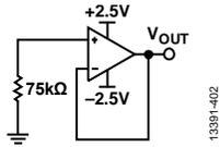
Figure 48. Current Noise Test Circuit (See Figure 20)
