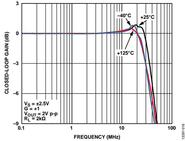
Figure 9. Large Signal Frequency Response for Various Temperatures
