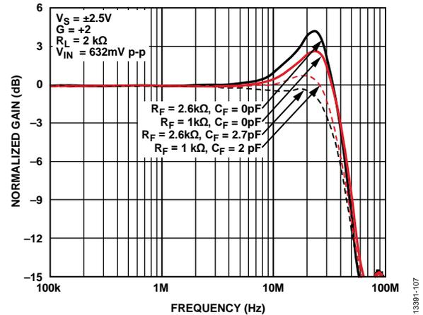
Figure 60. Peaking Mitigation in Large Signal Frequency Response
