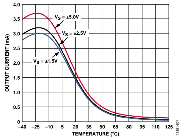
Figure 45. Sleep Mode Output Current vs. Temperature
