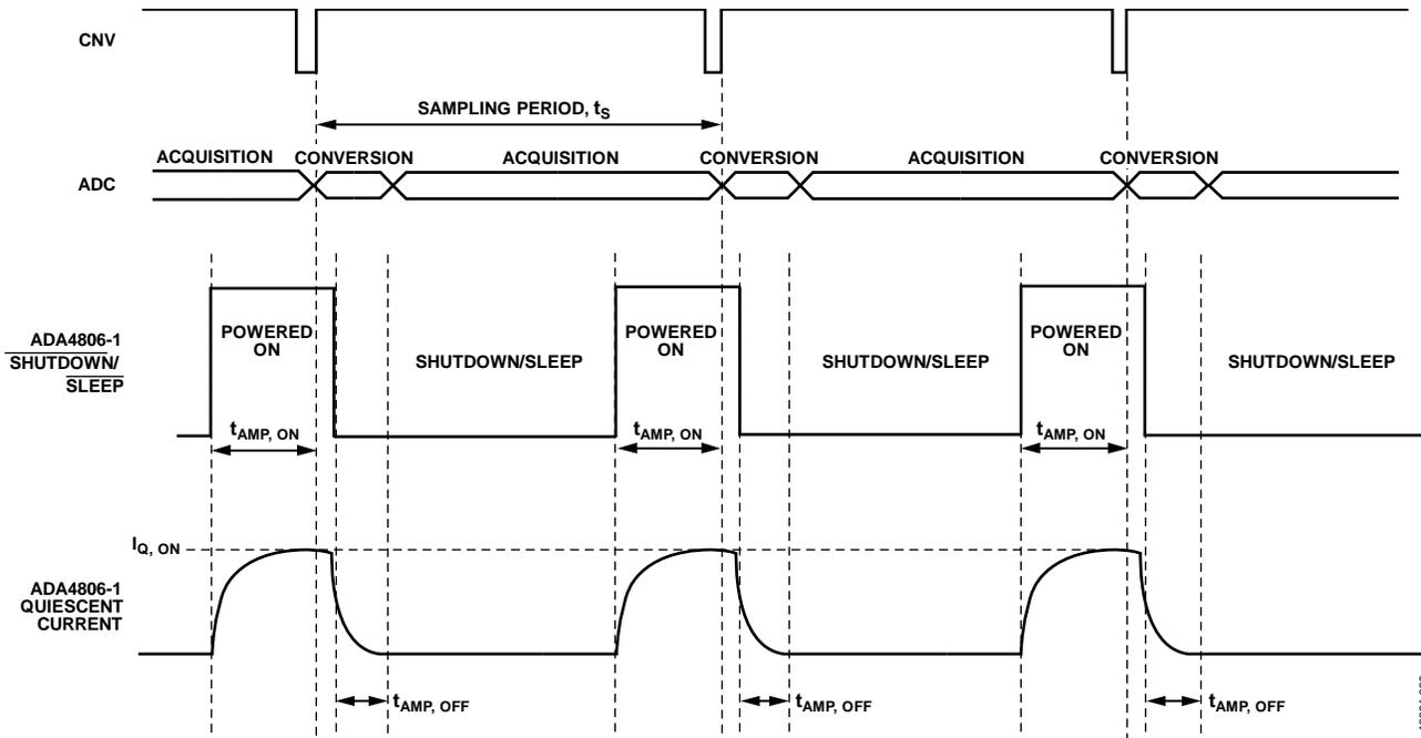
Figure 63. Timing Waveforms
