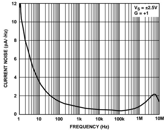
Figure 20. Current Noise vs. Frequency (See Figure 48)
