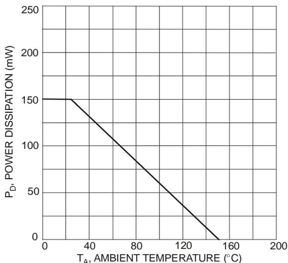
Fig. 1 Power Derating Curve, Total Package (Note 5)
