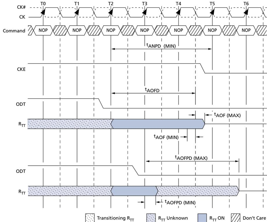
Figure 85: ODT Turn-On Timing When Entering Power-Down Mode
