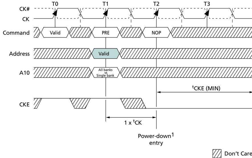
Note: 1. The earliest precharge power-down entry may occur is at T2, which is  $1 \times t_{CK}$  after the PRECHARGE command. Precharge power-down entry occurs prior to  $t_{RP}$  (MIN) being satisfied.
