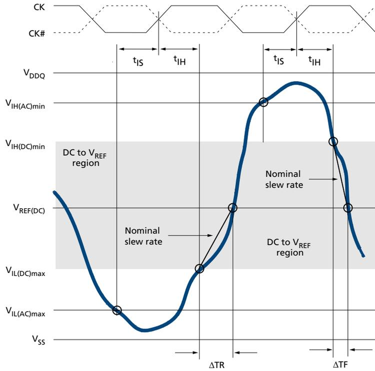
**Figure 26: Tangent Line for  $t_{IH}$**
