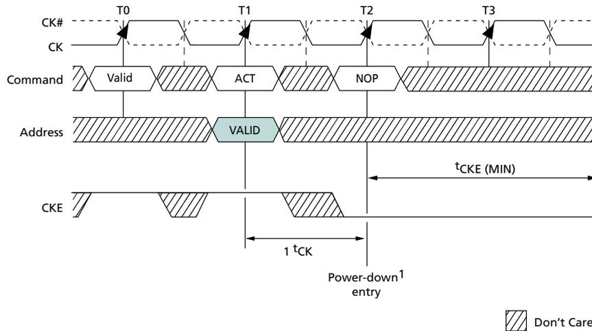
Note: 1. The earliest active power-down entry may occur is at T2, which is  $1 \times t_{CK}$  after the ACTIVATE command. Active power-down entry occurs prior to  $t_{RCD}(\text{MIN})$  being satisfied.
