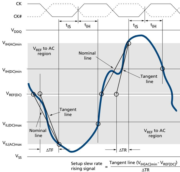
**Figure 25: Nominal Slew Rate for  $t_{IH}$**
