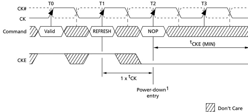
Note: 1. The earliest precharge power-down entry may occur is at T2, which is  $1 \times t_{CK}$  after the REFRESH command. Precharge power-down entry occurs prior to  $t_{RFC}(\text{MIN})$  being satisfied.
