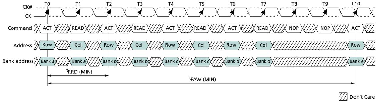
Note: 1. DDR2-533 (-37E, x4 or x8),  $t_{CK} = 3.75\text{ns}$ ,  $BL = 4$ ,  $AL = 3$ ,  $CL = 4$ ,  $t_{RRD}(\text{MIN}) = 7.5\text{ns}$ ,  $t_{FAW}(\text{MIN}) = 37.5\text{ns}$ .
