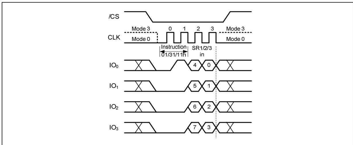
Figure 9b. Write Status Register-1/2/3 Instruction (QPI Mode)
