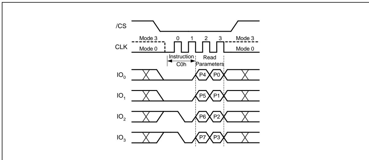
Figure 48. Set Read Parameters Instruction (QPI Mode only)
