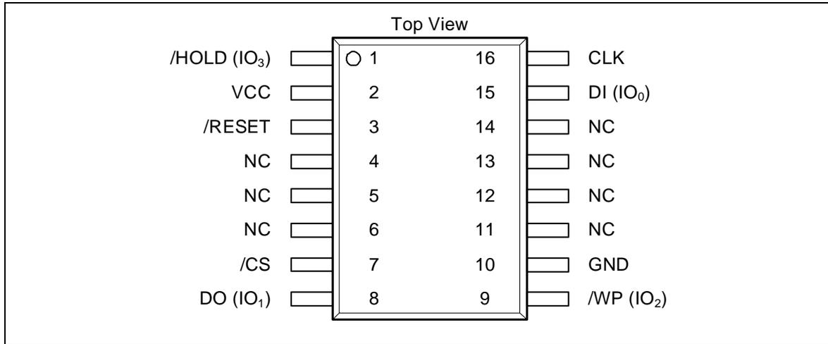
Figure 1b. W25Q256FV Pin Assignments, 16-pin SOIC 300-mil (Package Code F)
