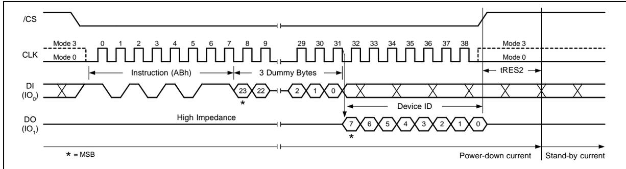
Figure 38c. Release Power-down / Device ID Instruction (SPI Mode)
