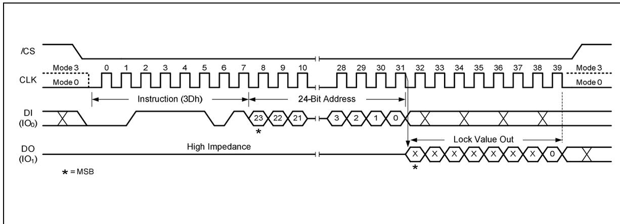
Figure 54a. Read Block Lock Instruction (SPI Mode)
