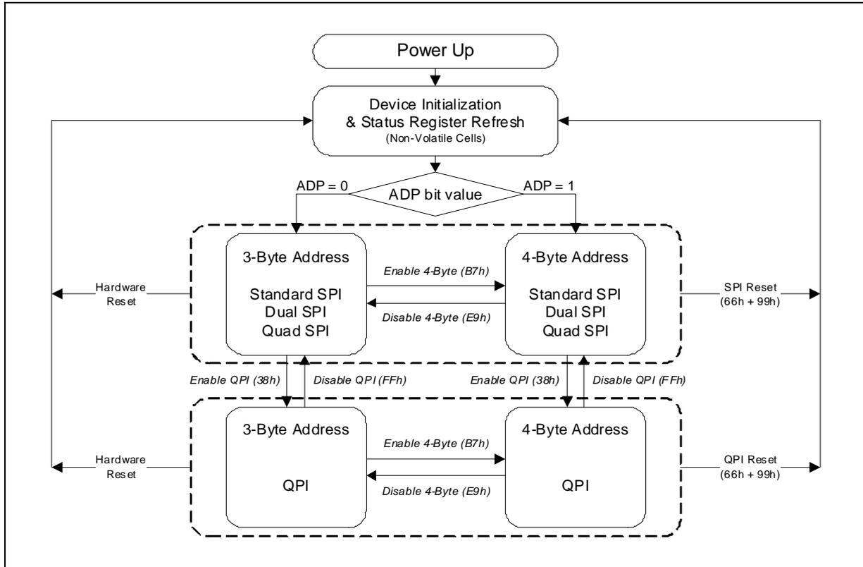
Figure 3. W25Q256FV Serial Flash Memory Operation Diagram
