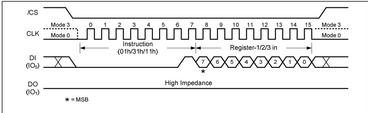
Figure 9a. Write Status Register-1/2/3 Instruction (SPI Mode)
