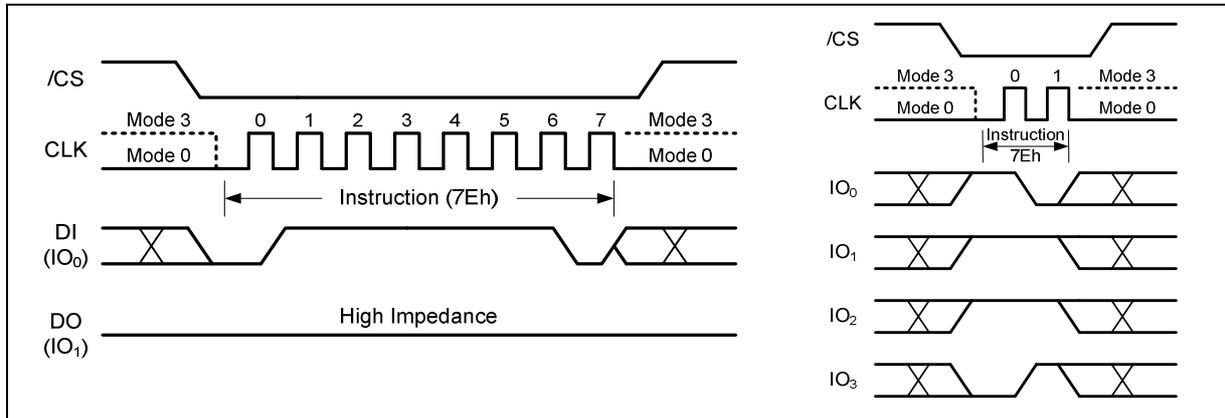
Figure 55. Global Block Lock Instruction for SPI Mode (left) or QPI Mode (right)
