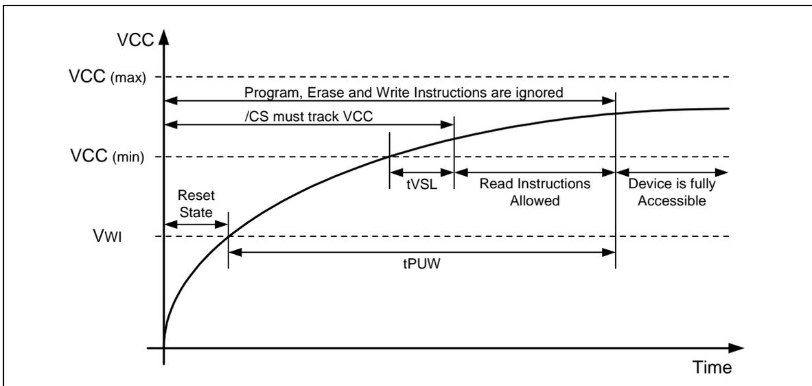
Figure 58. Power-up Timing and Voltage Levels
