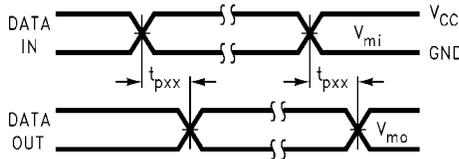
FIGURE 2. Waveform for Inverting and Non-Inverting Functions
