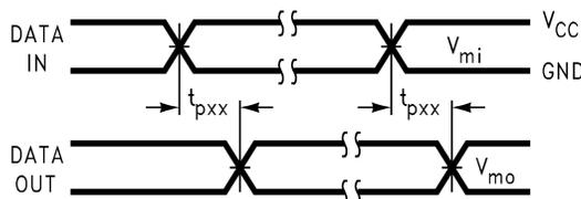
FIGURE 6. Waveform for Inverting and Non-Inverting Functions
