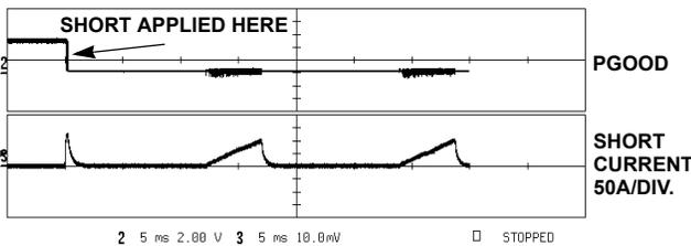
HICUP MODE. SUPPLY POWERED BY ATX SUPPLY
