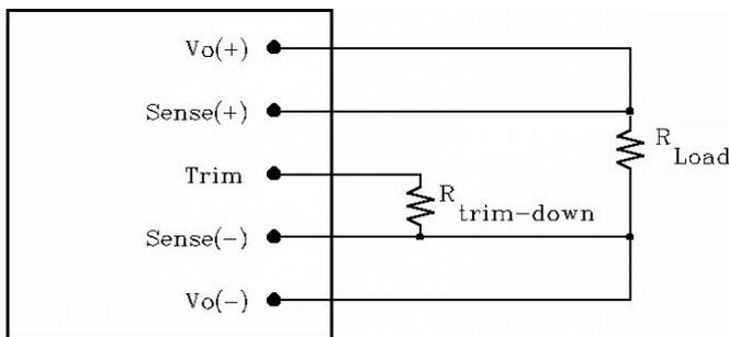
**Figure 18:** Circuit configuration for trim-down (decrease output voltage)
