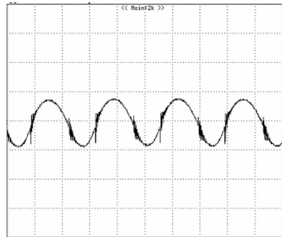
**Figure 11:** Input Terminal Ripple Current,  $i_c$ , at full rated output current and nominal input voltage with  $12\mu H$  source impedance and  $33\mu F$  electrolytic capacitor (200 mA/div, 1us/div)
