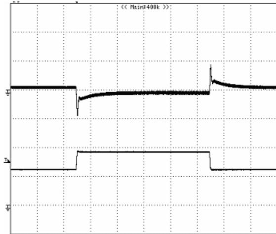
**Figure 9:** Output voltage response to step-change in load current (75%-50%-75% of  $I_o$ , max;  $di/dt = 1.0A/\mu s$ ). Load cap:  $100\mu F$  tantalum capacitor and  $1\mu F$  ceramic capacitor. Top Trace:  $V_{out}$  (50mV/div, 200us/div), Bottom Trace:  $I_{out}$  (10A/div). Scope measurement should be made using a BNC cable (length shorter than 20 inches). Position the load between 51 mm to 76 mm (2 inches to 3 inches) from the module
