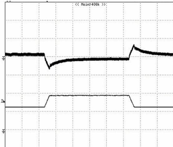
**Figure 8:** Output voltage response to step-change in load current (75%-50%-75% of  $I_o$ , max;  $di/dt = 0.1A/\mu s$ ). Load cap:  $10\mu F$  tantalum capacitor and  $1\mu F$  ceramic capacitor. Top Trace:  $V_{out}$  (50mV/div, 200us/div), Bottom Trace:  $I_{out}$  (10A/div). Scope measurement should be made using a BNC cable (length shorter than 20 inches). Position the load between 51 mm to 76 mm (2 inches to 3 inches) from the module
