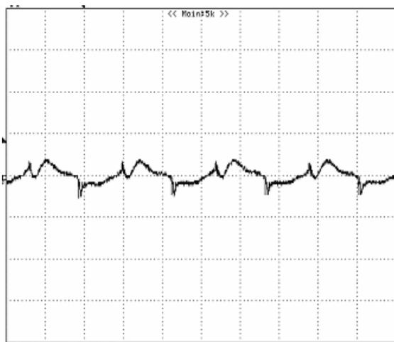
**Figure 14:** Output voltage ripple at nominal input voltage and rated load current ( $I_o=25\text{A}$ ) (50 mV/div, 1  $\mu\text{s}$ /div)
