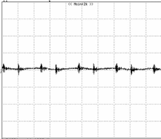
**Figure 12:** Input reflected ripple current,  $i_s$ , through a  $12\mu\text{H}$  source inductor at nominal input voltage and rated load current (20 mV/div, 1  $\mu\text{s}$ /div)
