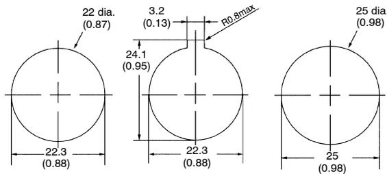
For 25 mm-dia. holes, always use 25 mm-dia. Rings. (Since the cutout dimensions are large, IP65 cannot be guaranteed unless 25-dia. Rings are used.)
