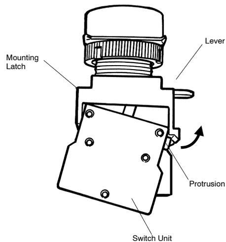
**Removing the Switch Unit**
