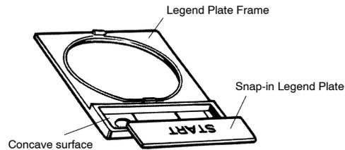
To easily remove the Snap-in Legend Plate from the Legend Plate Frame mounted to the panel, insert a Tool with a thin tip into the space between the Snap-in Legend Plate and the Legend Plate Frame.
