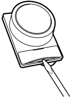
The Snap-in Legend Plate is easily removed by pressing the Snap-in Legend Plate from the back of the Legend Plate Frame.
