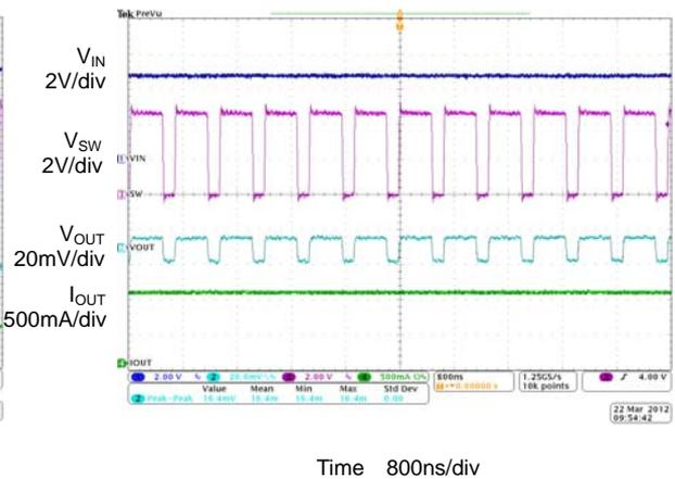
Figure 17.  $V_{OUT}$  Ripple
