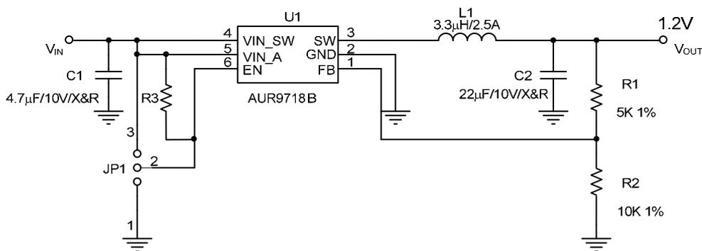
Figure 31. The Evaluation Board Schematic
