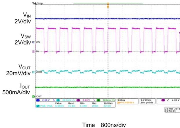
Figure 16.  $V_{OUT}$  Ripple
