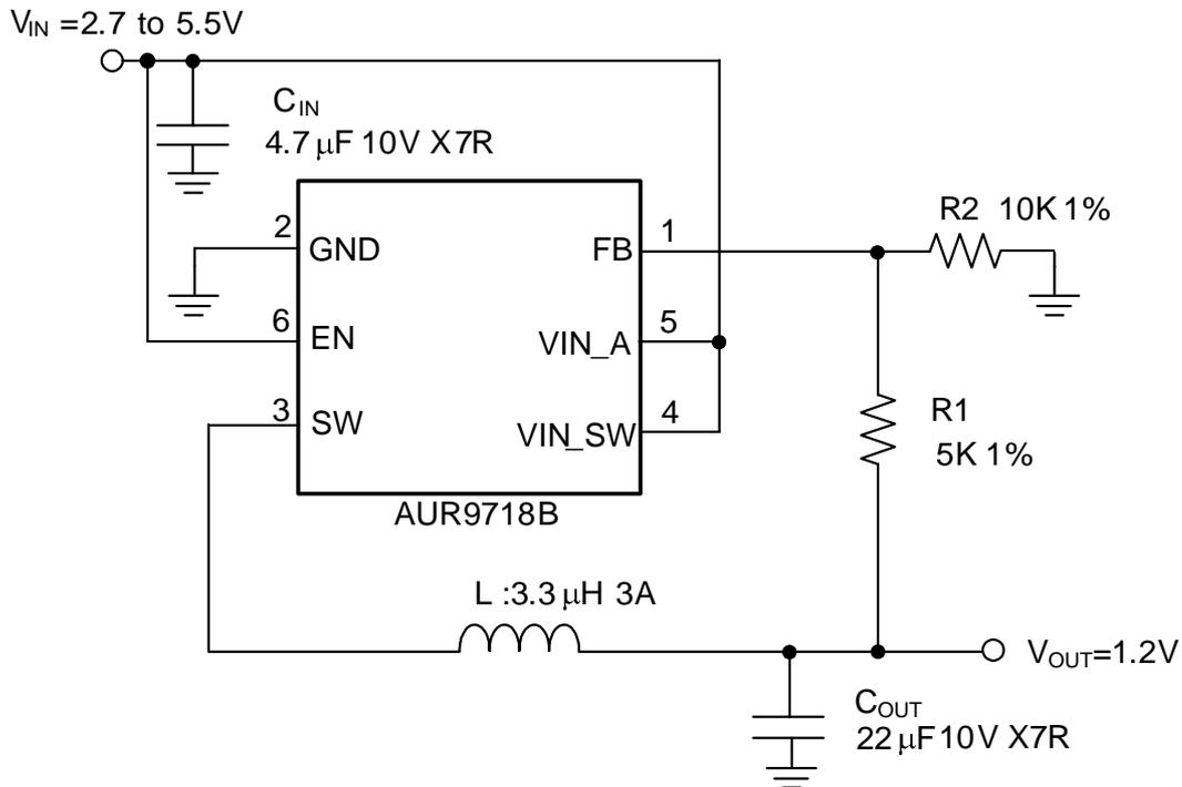
Note 2:  $V_{OUT} = V_{FB} \times \left(1 + \frac{R_1}{R_2}\right)$
