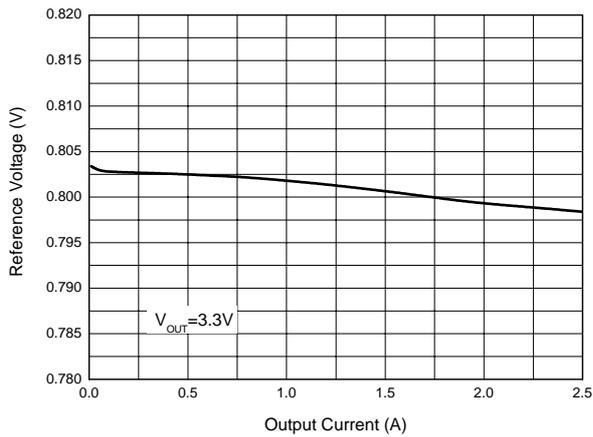
Figure 14. Reference Voltage vs. Output Current
