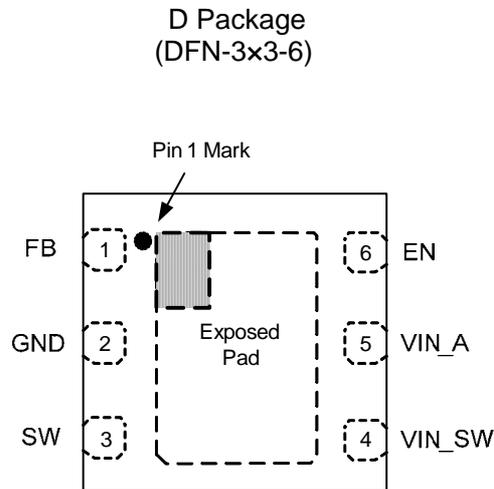
Figure 2. Pin Configuration of AUR9718B (Top View)
