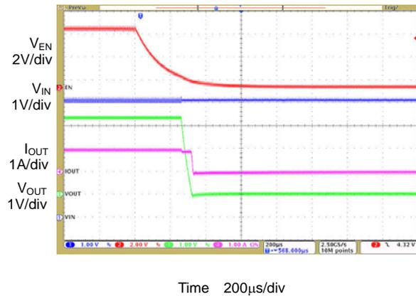
Figure 24. EN Pin H to L
