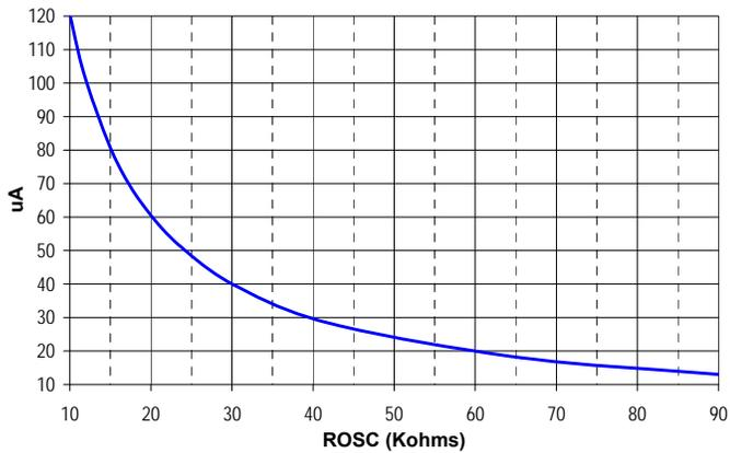
**Figure 16: I(REGSET) CURRENT versus ROSC**
