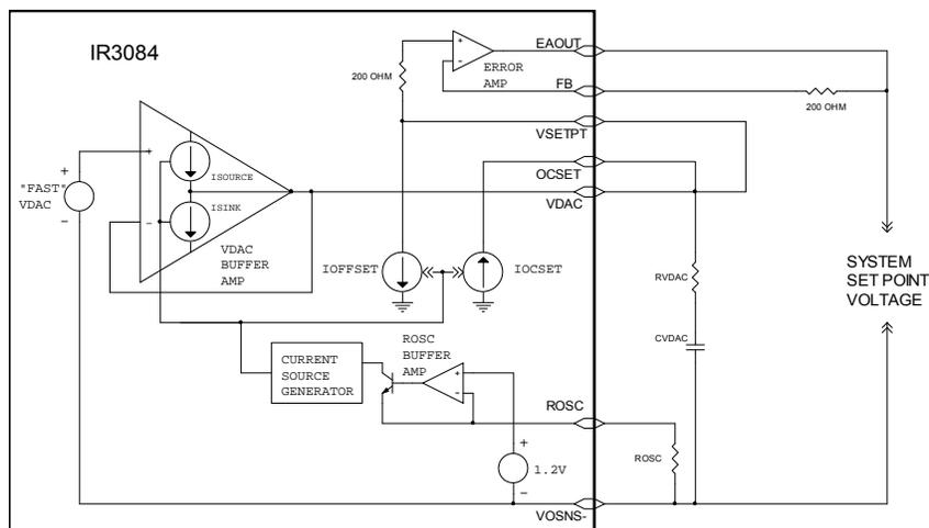
**Figure 1 – System Set Point Test Circuit**
