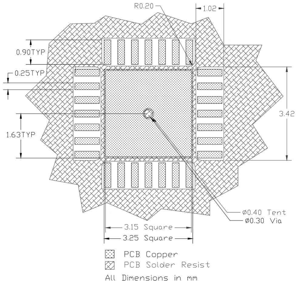
**PCB METAL AND COMPONENT PLACEMENT**
