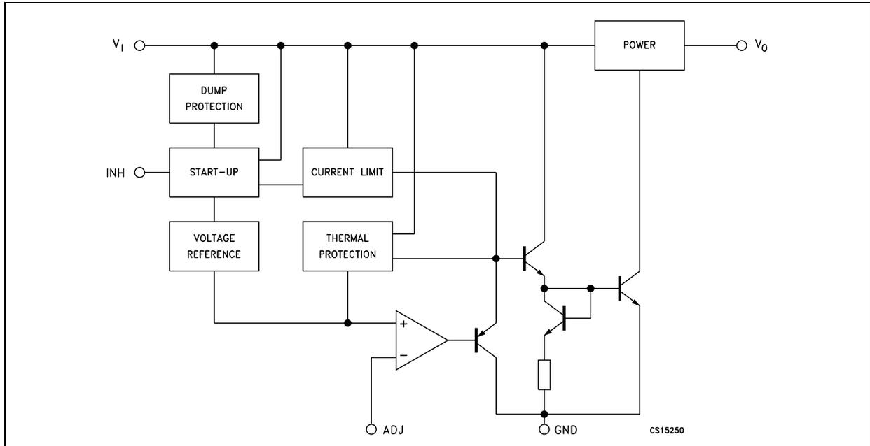
Figure 2. Schematic diagram for fixed version
