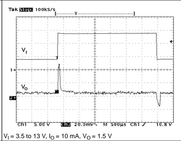
Figure 19. Load transient
