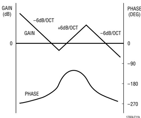
Figure 11B. Type 3 Amplifier Transfer Function
