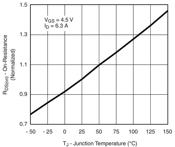
$T_J$  - Junction Temperature ( $^\circ\text{C}$ )
