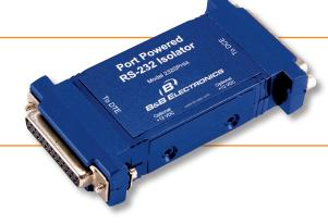
The 232SPHI4 isolates and protects RS-232 equipment from lightning surges, accidental high voltage shorts, and ground loops. RS-232 data signals at up to 115.2K bps as well as the RTS and CTS handshake lines are supported. The 232SPHI4 provides 4000 Volts of isolation between sides, and maintains creepage and air clearances required for double or reinforced insulation by IEC 60601-1.
