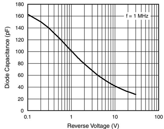
Fig. 6 - Diode Capacitance vs. Reverse Voltage
