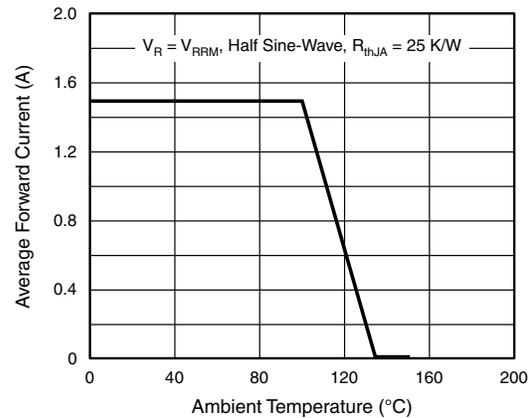
Fig. 2 - Max. Average Forward Current vs. Ambient Temperature
