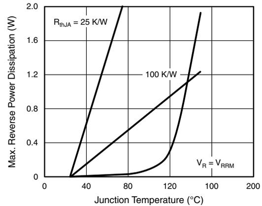
Fig. 5 - Max. Reverse Power Dissipation vs. Junction Temperature
