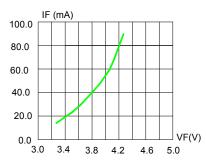
FIG.1 FORWARD CURRENT VS. FORWARD VOLTAGE.
