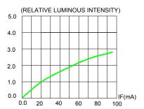
FIG.2 RELATIVE LUMINOUS INTENSITY VS. FORWARD CURRENT
