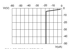
FIG.3 REVERSE CURRENT VS. REVERSE VOLTAGE.
