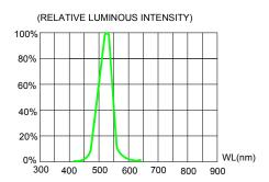
FIG.5 RELATIVE LUMINOUS INTENSITY VS. WAVELENGTH.
