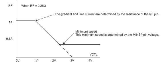
The current flowing to the motor and the control characteristics are determined by adjusting the resistance of the RF resistor.
