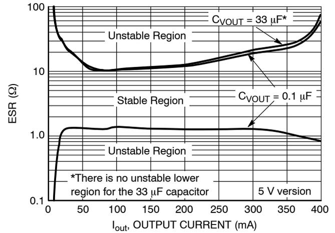
Figure 8. Output Stability with Output Capacitor Change
