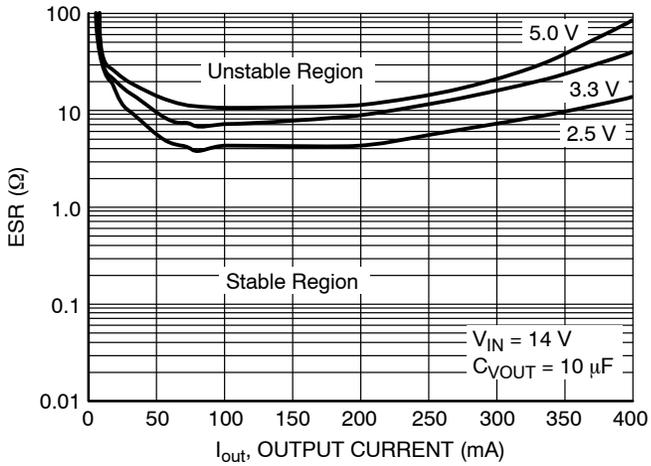
Figure 7. Output Stability with Output Voltage Change
