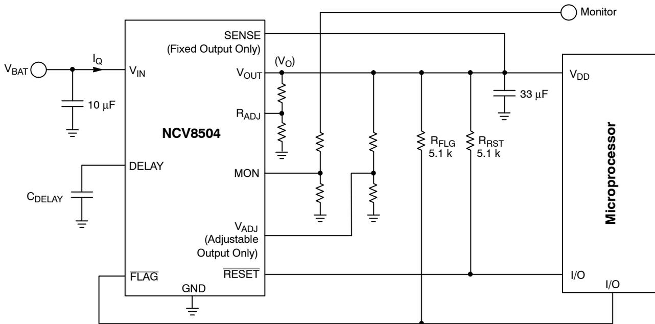
Figure 1. Application Diagram
