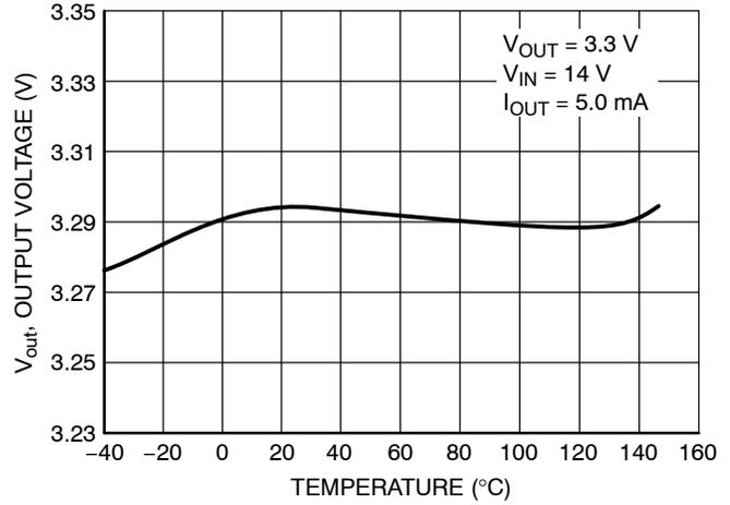
Figure 4. 3.3 V Output Voltage vs Temperature
