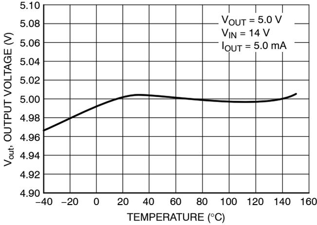
Figure 3. 5 V Output Voltage vs Temperature
