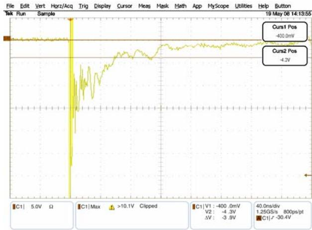
**Figure 2. ESD Clamping Voltage Screenshot
