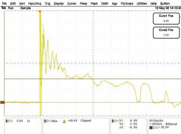
**Figure 1. ESD Clamping Voltage Screenshot
