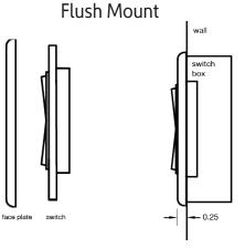
For flush mount, mount the switch without the backplate into either a standard electrical switch box or a low voltage mounting bracket using included screws.
