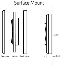
For surface mount, attach included backplate to the wall using screws or adhesive.
