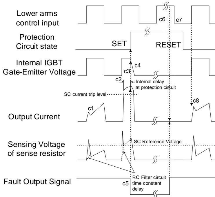
**Figure 13. Short-Circuit Current Protection (Low-Side Operation only)**
