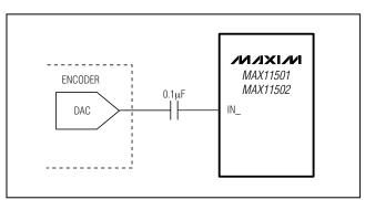
Figure 3. Simple AC-Coupling for Unipolar Signals (Y, R, G, B)
