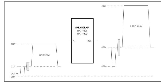
Figure 2. Typical DC-Coupled Signal
