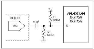
Figure 4. AC-Coupling for Bipolar Signals (Pb, Pr)
