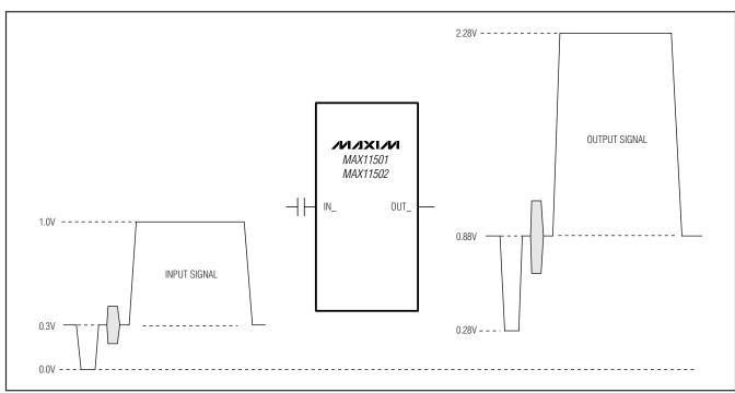
Figure 1. Typical AC-Coupled Signal
