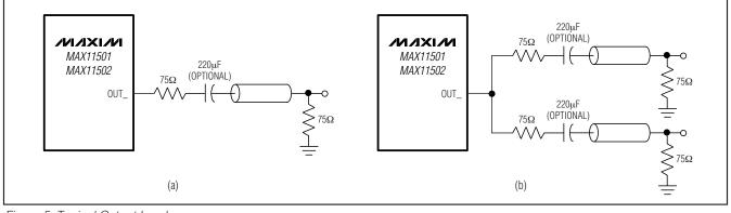
Figure 5. Typical Output Loads
