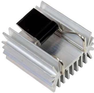
Ohmite's R2 Series (patent pending) heatsink provides a large surface area along with our C Series clipping mechanism to attach to a TO-220, TO-247, or TO-264 package. The self-aligning features of the clip assure secure attachment and enhanced thermal performance. Because no screws are required for device mounting, additional fins can be added to the rear side of the heatsink for increased total surface area in a more compact space.
