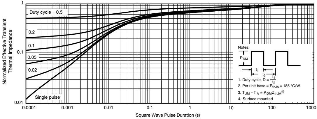
**Normalized Thermal Transient Impedance, Junction-to-Ambient (on 1" x 1" FR4 board with maximum copper)**
