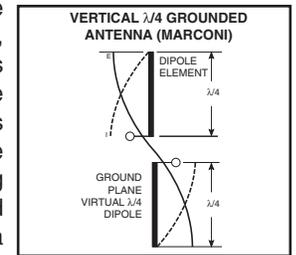
Figure 21: Dipole Antenna
