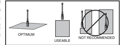
3. If an internal antenna is to be used, keep it away from other metal components, particularly large items like transformers, batteries, and PCB tracks and groundplanes. In many cases, the space around the antenna is as important as the antenna itself. Objects in close proximity to the antenna can cause direct detuning, while those farther away will alter the antenna's symmetry.
