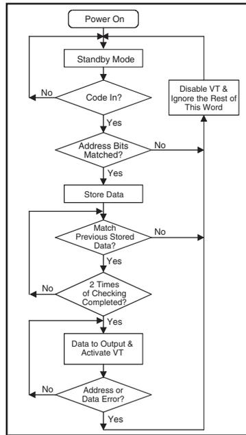
Figure 9: Decoder Flowchart
