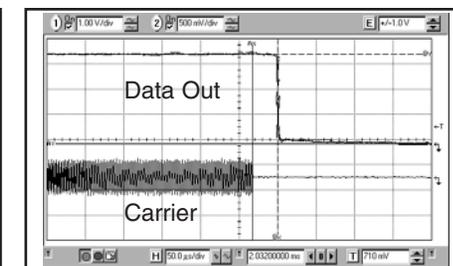
Figure 6: Receiver Turn-off Time
