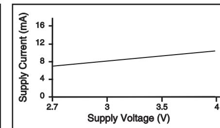
Figure 4: Consumption vs. Supply Voltage
