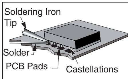
Figure 18: Soldering Technique
