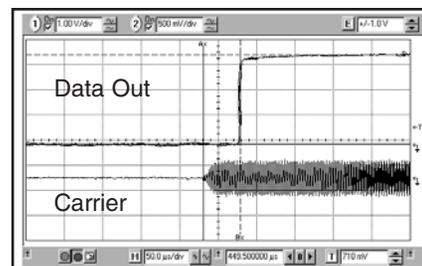
Figure 5: RF In vs. Receiver Response Time
