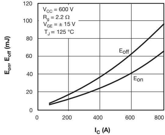
Fig. 3 - IGBT Switching Loss vs. Collector Current
