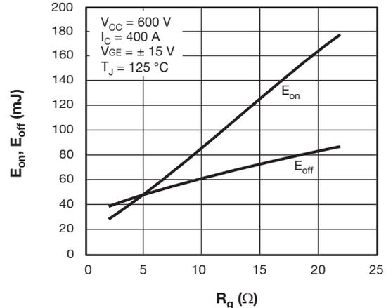
Fig. 4 - IGBT Switching Loss vs. Gate Resistor
