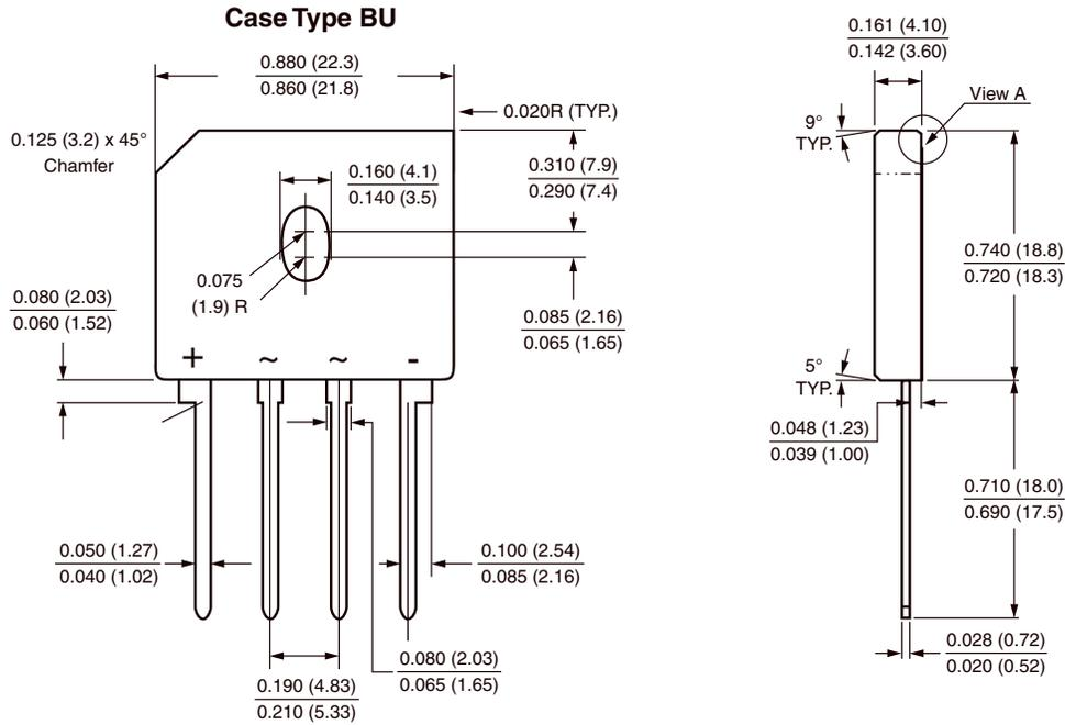
Polarity shown on front side of case, positive lead beveled corner
