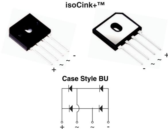
\* Tested to UL standard for safety electrically isolated semiconductor devices. UL 1557 4th edition. Dielectric tested to maximum case, storage and junction temperature to 150 °C to withstand 1500 V. Epoxy meets UL 94 V-0 flammability rating.
