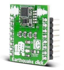
**Earthquake click** carries D7S, the world's smallest high-precision seismic sensor from Omron. The click is designed to run on either 3.3V or 5V power supply. It communicates with the target MCU over I2C interface, with additional functionality provided by the following pins on the mikroBUS<sup>TM</sup> line: PWM, INT, CS.
