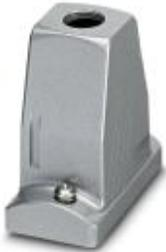
HEAVYCON ADVANCE STA sleeve housing B6, with screw locking, height 100 mm, with 1x M20 thread, straight cable outlet, with M6 x 18 hexagonal socket-head screws made of high-grade steel in acc. with DIN EN ISO 4762
