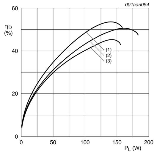
$V_{DS} = 32\text{ V}; I_{Dq} = 100\text{ mA}; t_p = 100\text{ }\mu\text{s}; \delta = 20\text{ }\%$ .
