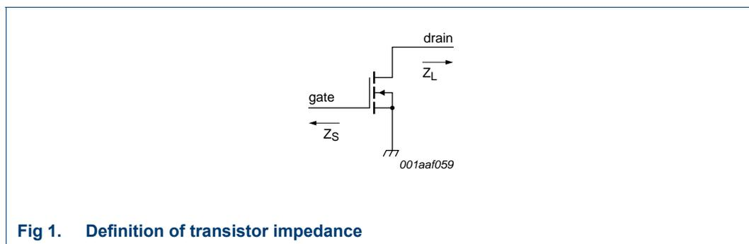
Fig 1. Definition of transistor impedance
