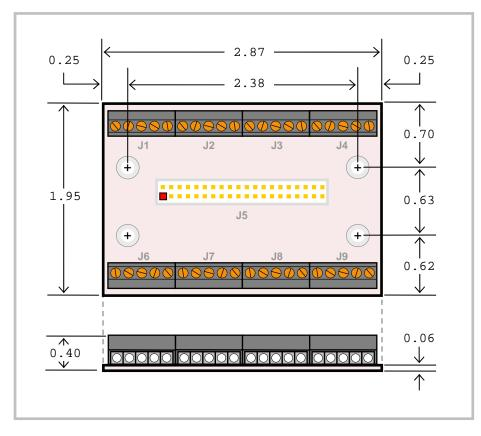
Figure 7. CBR-4004 Dimensions and Mounting Holes
