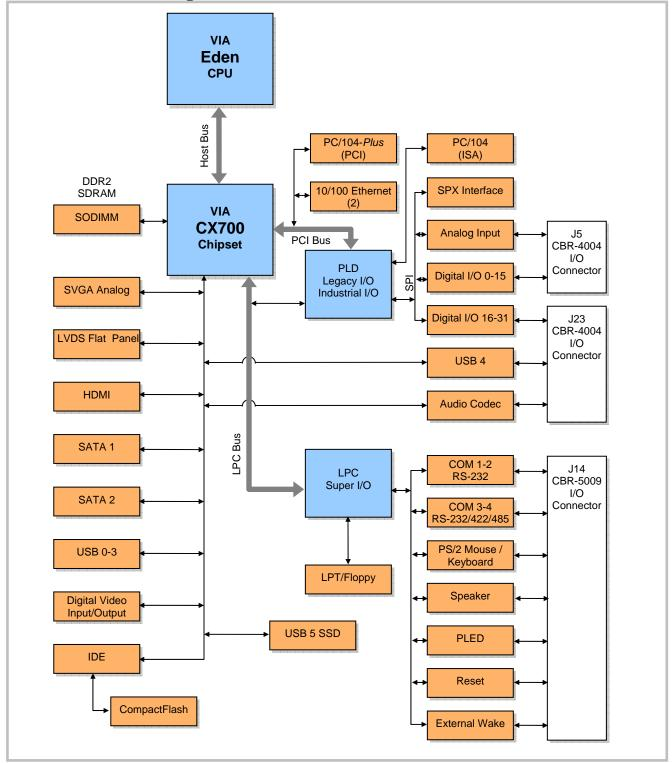
Figure 1. EBX-22 Block Diagram
