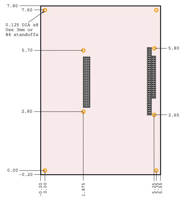
Figure 4. EBX-22 Dimensions and Mounting Holes (Not to scale. All dimensions in inches.)
