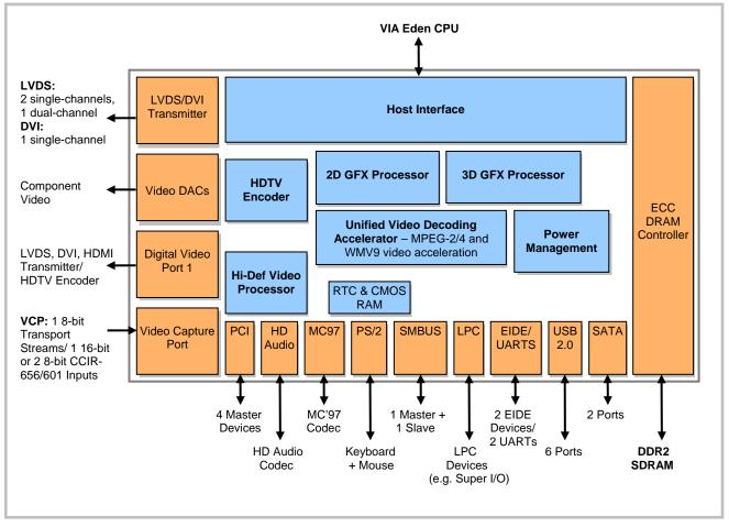
Figure 2. CX700M Block Diagram
