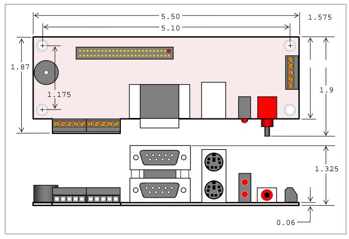
Figure 6. CBR-5009 Dimensions and Mounting Holes
