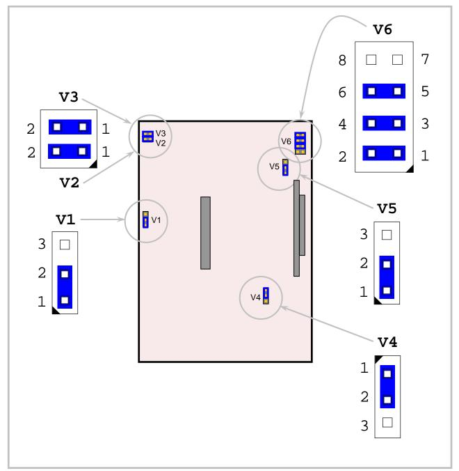
Figure 12. Jumper Block Locations
