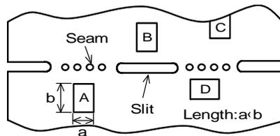
Products (A, B, C, D) shall be located carefully so that products are not subject to the mechanical stress due to warping the board. Because they may be subjected the mechanical stress in order of A>C>B≧D.
