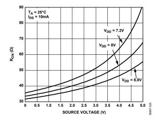
Figure 7.  $R_{ON}$  vs. Source Voltage,  $V_{DD} = 8 V \pm 10\%$
