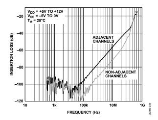
Figure 21. Crosstalk vs. Frequency
