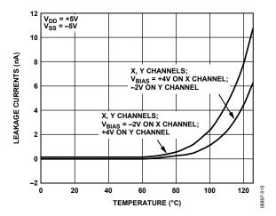
Figure 12. Off Leakage vs. Temperature, Dual ±5 V Supplies
