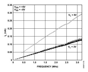
Figure 22. Digital Current (IL) vs. Frequency
