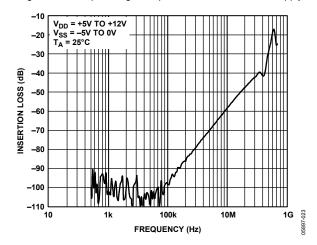
Figure 20. Off Isolation vs. Frequency
