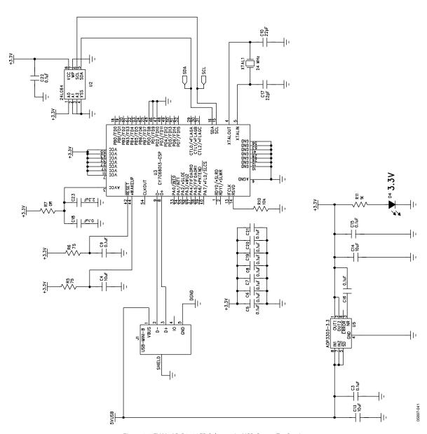
Figure 36. EVAL-ADG2188EB Schematic, USB Controller Section
