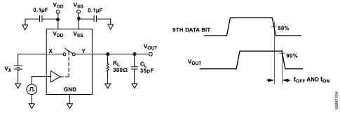
Figure 28. Switching Times, ton, toff
