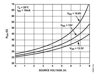
Figure 6.  $R_{ON}$  vs. Supplies,  $V_{DD} = 12 V \pm 10\%$
