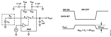
Figure 29. Charge Injection
