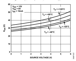
Figure 9.  $R_{ON}$  vs. Temperature,  $V_{DD} = 12 V$
