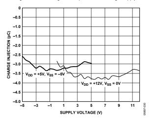
Figure 15. Charge Injection vs. Supply Voltage
