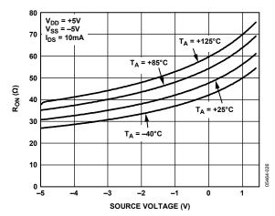
Figure 8.  $R_{ON}$  vs. Temperature, Dual  $\pm 5$  V Supplies
