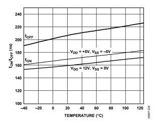
Figure 16. ton/toff Times vs. Temperature
