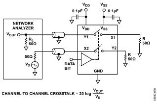
Figure 32. Channel-to-Channel Crosstalk
