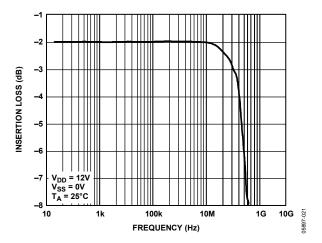
Figure 18. Individual Inputs to Individual Outputs Bandwidth, 12 V Single Supply
