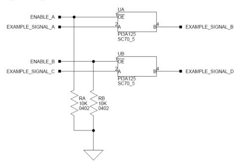
Figure 3-2: Example of Individual FET Switches
