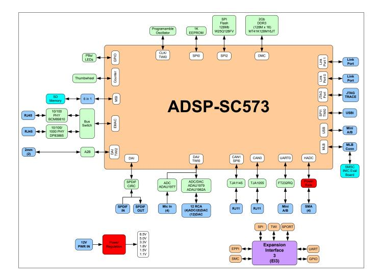
Figure 3-1: Block Diagram
