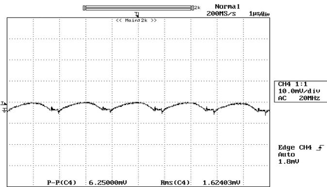
Figure 9: Output ripple & noise at 12Vin, 1.5V/20A out
