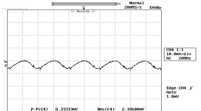
Figure 10: Output ripple & noise at 12Vin, 2.5V/20A out
