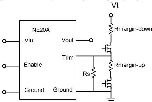
**Figure 22:** Circuit configuration for output voltage margining
