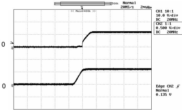
Figure 13: Turn on delay time at 12Vin, 0.59V/20A out
