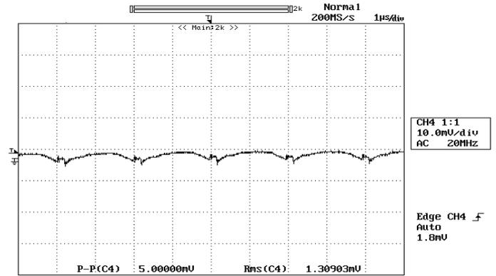
Figure 8: Output ripple & noise at 12Vin, 0.9V/20A out
