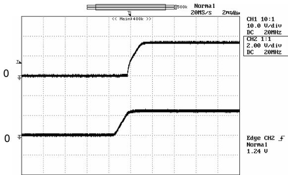
Figure 15: Turn on delay time at 12Vin, 3.3V/20A out
