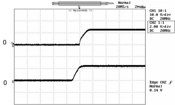
Figure 14: Turn on delay time Remote On/Off, 2.5V/20A out
