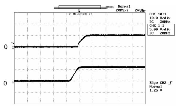
Figure 16: Turn on delay time at Remote On/Off, 5.0V/20A out
