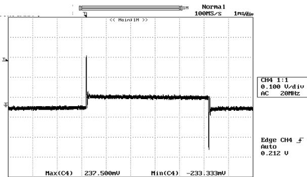
Figure 17: Typical transient response to step load change at 5A/μs
