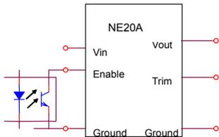
**Figure 20:** Enable input drive circuit example with isolation.
