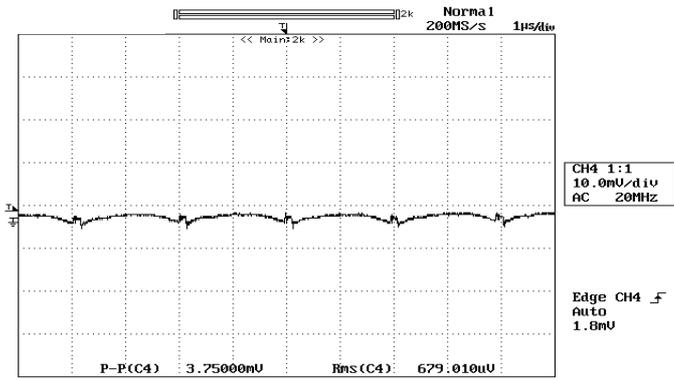
Figure 7: Output ripple & noise at 12Vin, 0.59V/20A out
