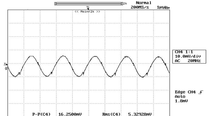
Figure 12: Output ripple & noise at 12Vin, 5.0V/20A out
