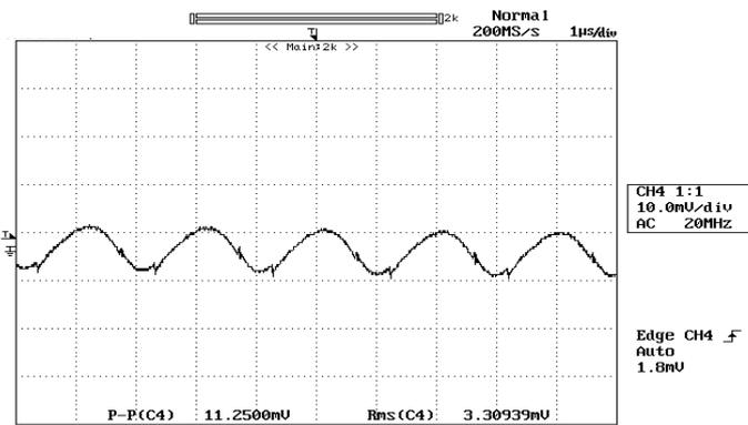
Figure 11: Output ripple & noise at 12Vin, 3.3V/20A out
