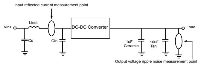
$$C_s = 270\mu\text{F} \times 1, L_{test} = 2\mu\text{H}, C_{in} = 270\mu\text{F} \times 1$$
