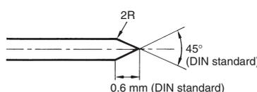
The shape of the Plug contact tip is based on the DIN standard dimensions, however, a small radius, R, has been introduced between the shaft and the tip. This results in less force being required for insertion.
