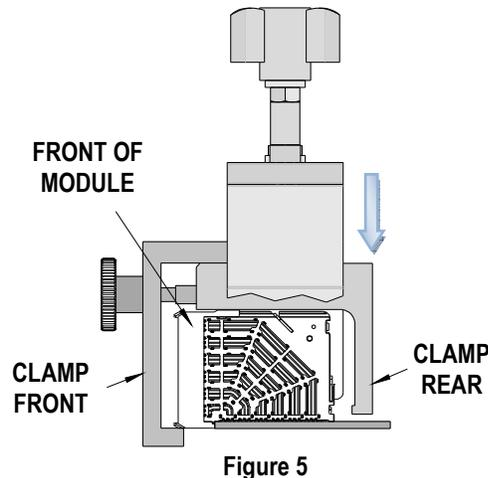
4. Slide the clamp front onto the bottom lip of the front module by turning the thumb screw clockwise. See Figure 6.
