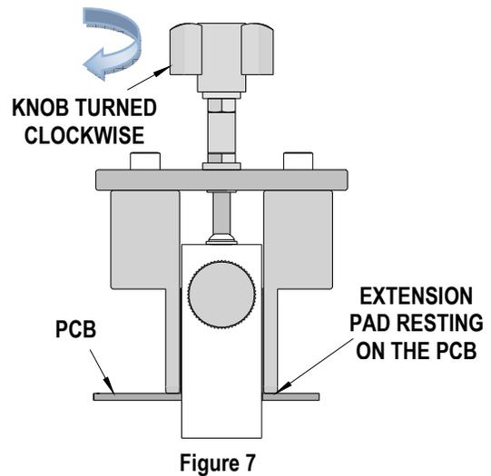
6. Make sure the clamp front and rear are in position before lifting the Daughtercard module off the PCB.
