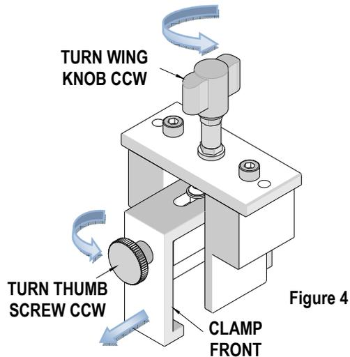
2. Turn the thumb screw counter clockwise so the clamp front can slide forward shown in Figure 4.
