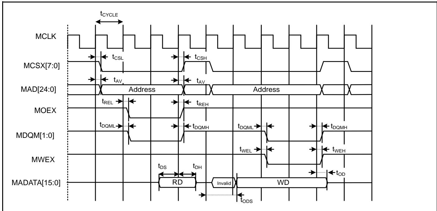
**Multiplexed Bus Access Asynchronous SRAM Mode**
