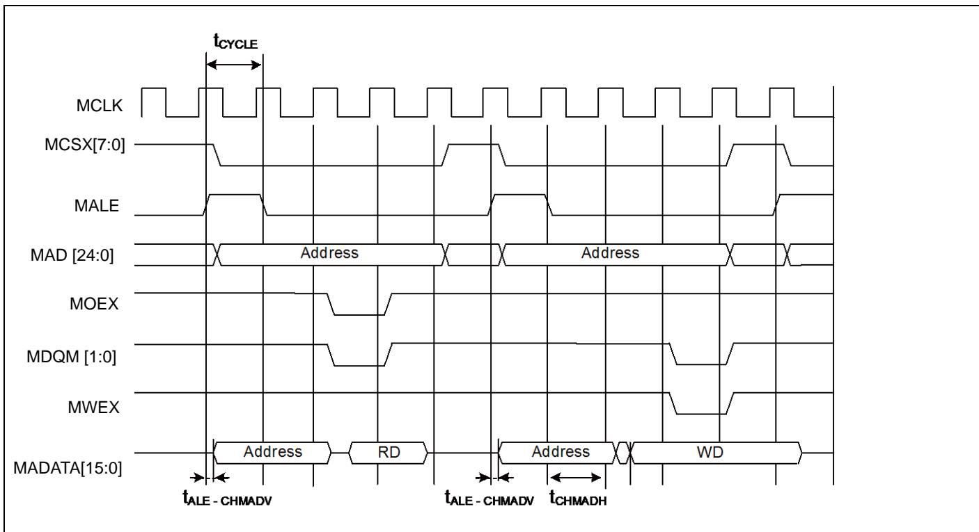
**Multiplexed Bus Access Synchronous SRAM Mode**
