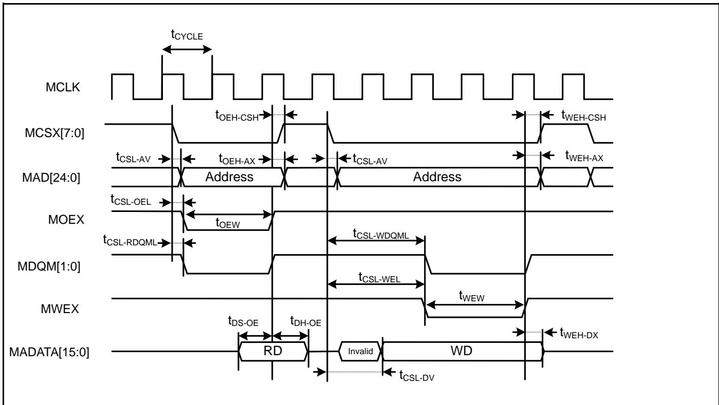
**Separate Bus Access Synchronous SRAM Mode**
