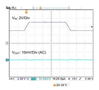
Figure 22. Line Transient (I<sub>OUT</sub>=500mA Slew Rate=0.2V/µs)
