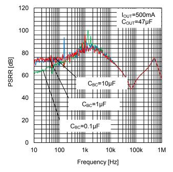
Figure 19. Power-Supply Rejection Ratio vs  $C_{BC}$
