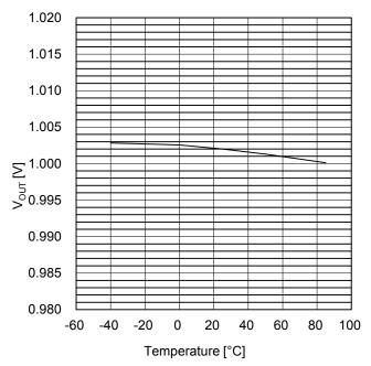
Figure 14. Output Voltage vs Temperature
