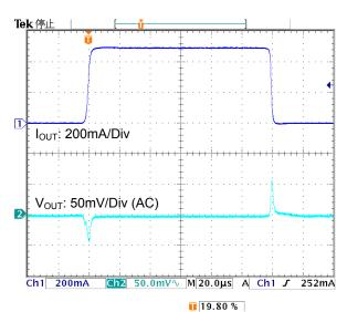
Figure 21. Load Transient (I<sub>OUT</sub>=0mA to 500mA)
