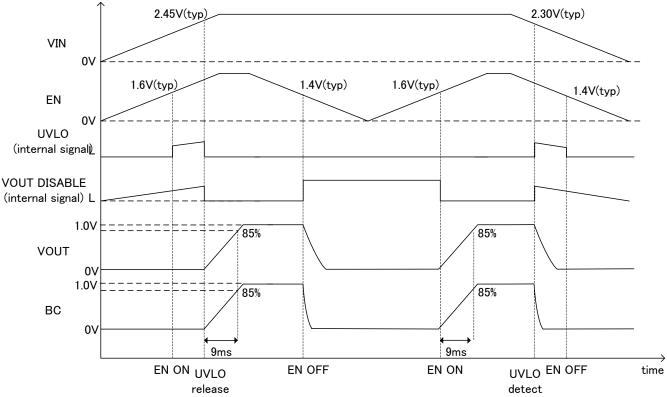
Figure 4. The Waveform During VIN/EN Rising and Falling (When at BC Capacitor 1µF and Output 1V Settings)
