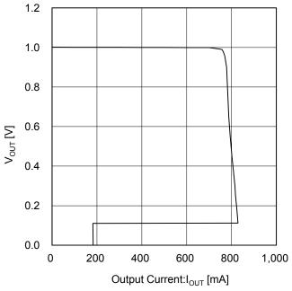
Figure 13. Output Voltage vs Output Current
