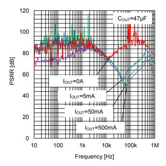
Figure 15. Power-Supply Rejection Ratio vs I<sub>OUT</sub>
