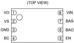
Figure 2. Pin Configuration
