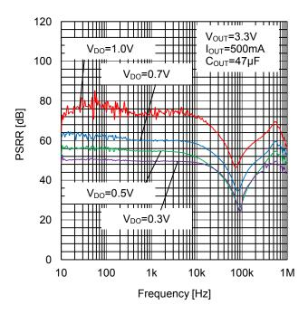
Figure 16. Power-Supply Rejection Ratio vs  $V_{\text{DO}}$
