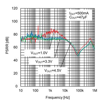
Figure 18. Power-Supply Rejection Ratio vs Vout
