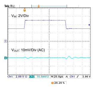
Figure 21. Line Transient (I<sub>OUT</sub>=500mA Slew Rate=1V/µs)
