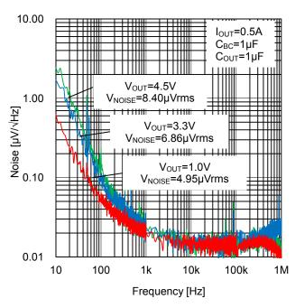
Figure 6. Noise vs V<sub>OUT</sub>
