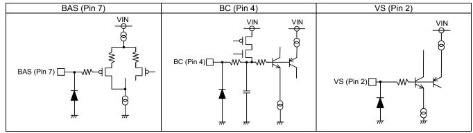
Figure 27. I/O Equivalence Circuits
