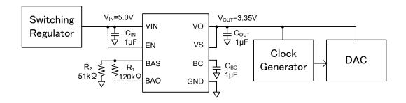
Figure 1. Basic Application Circuit Diagram (Vout=3.35V)
