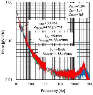
Figure 7. Noise vs I<sub>OUT</sub>
