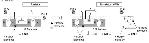
Figure 29. Example of Monolithic IC Structure
