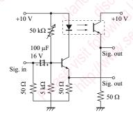
Measurement circuit of frequency characteristics
