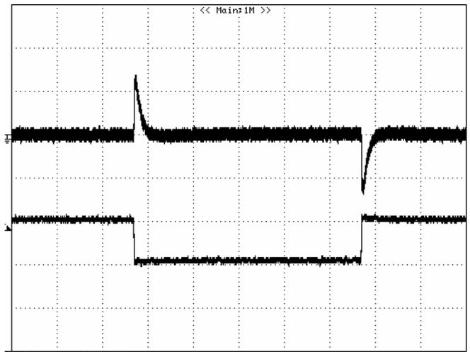
**Figure 9:** Output voltage response to step-change in load current (75%-50%-75% of  $I_{o, \max}$ ;  $di/dt = 2.5A/\mu s$ ). Load cap:  $47\mu F$ ,  $35m\Omega$  ESR solid electrolytic capacitor and  $1\mu F$  ceramic capacitor. Top Trace:  $V_{out}$  (0.1 V/div, 1ms/div), Bottom Trace:  $I_{out}$  (1A/div). Scope measurement should be made using a BNC cable (length shorter than 20 inches). Position the load between 51 mm to 76 mm (2 inches to 3 inches) from the module
