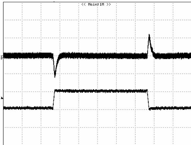
**Figure 8:** Output voltage response to step-change in load current (75%-50%-75% of  $I_{o, \max}$ ;  $di/dt = 0.01A/\mu s$ ). Load cap:  $10\mu F$  tantalum capacitor and  $1\mu F$  ceramic capacitor. Top Trace:  $V_{out}$  (0.1V/div, 1ms/div), Bottom Trace:  $I_{out}$  (1A/div). Scope measurement should be made using a BNC cable (length shorter than 20 inches). Position the load between 51 mm to 76 mm (2 inches to 3 inches) from the module
