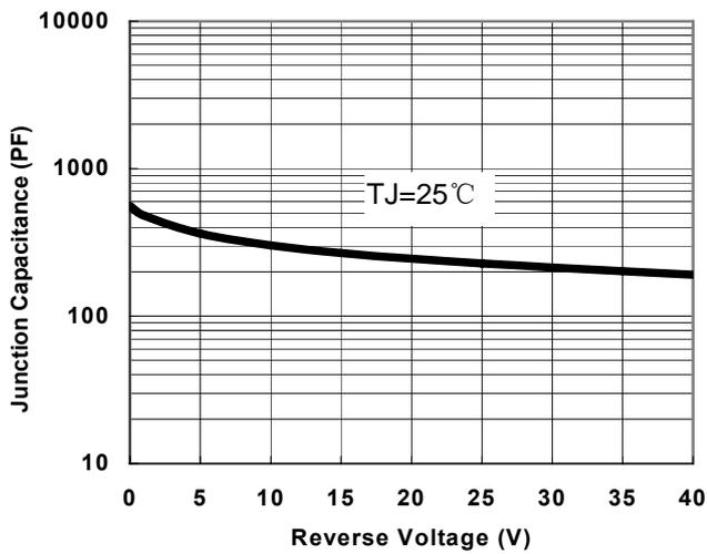
**Fig.1-Typical Junction Capacitance**
