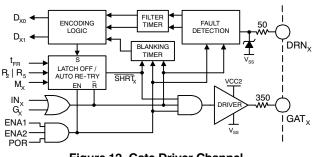
Figure 12. Gate Driver Channel
