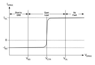
Figure 14. DRN<sub>X</sub> Bias and Fault Detection Zones
