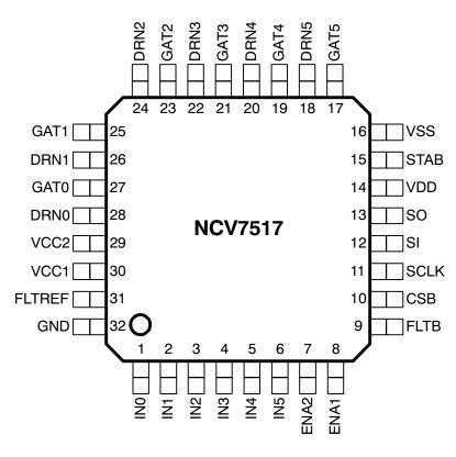
Figure 3. 32 Pin LQFP Pinout (Top View)
