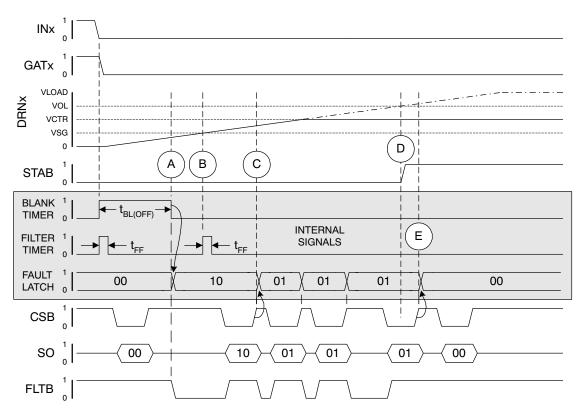
Figure 20. Short to GND/Open Load
