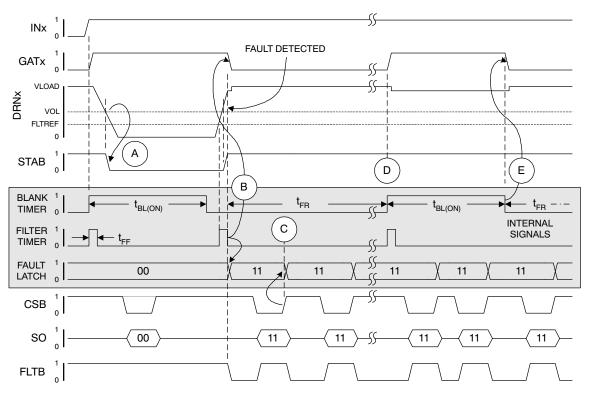
Figure 18. Shorted Load Detected
