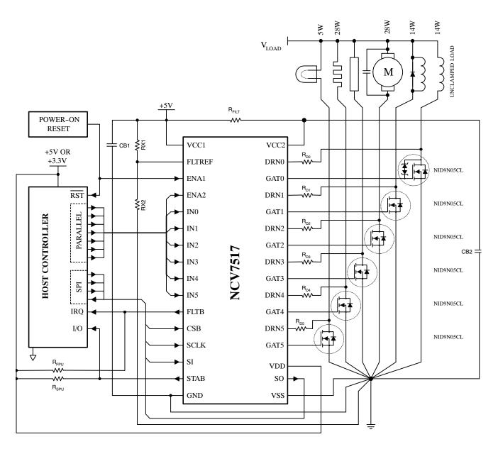
Figure 2. Application Diagram
