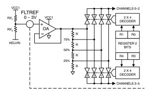
Figure 13. Shorted Load Reference Generator
