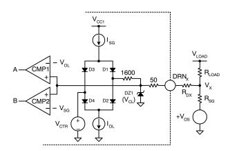
Figure 15. Short to GND/Open-Load Detection
