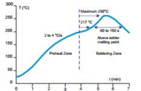
Fig. 3. Reflow Temperature Profile for Pb-free Soldering
