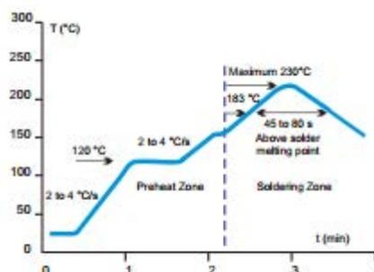
Fig. 2. Infrared Reflow Temperature Profile for Pb-containing Soldering
